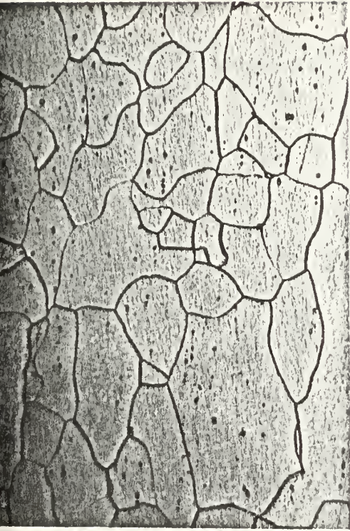
FIG. 26 AT 540°C FOR 30 HOURS (ROCKWELL 30T 33.7)
